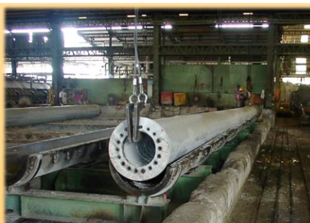
脫模 (PILE OUT OF FROM MOLD)
